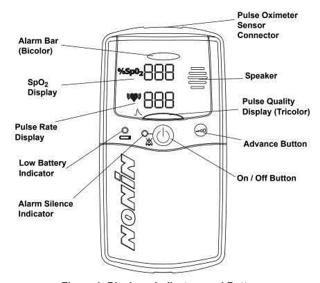
Figure 1: Displays, Indicators and Buttons
