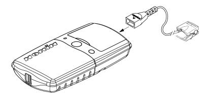
Figure 4: Connecting a Sensor
