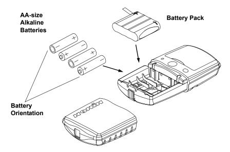
Figure 3: Installing Batteries
